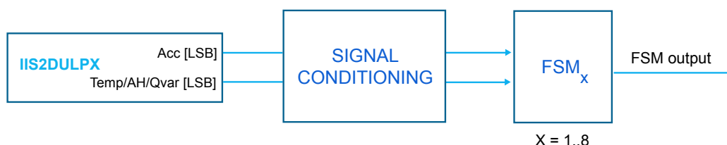
Figure 12. State machine in the IIS2DULPX
